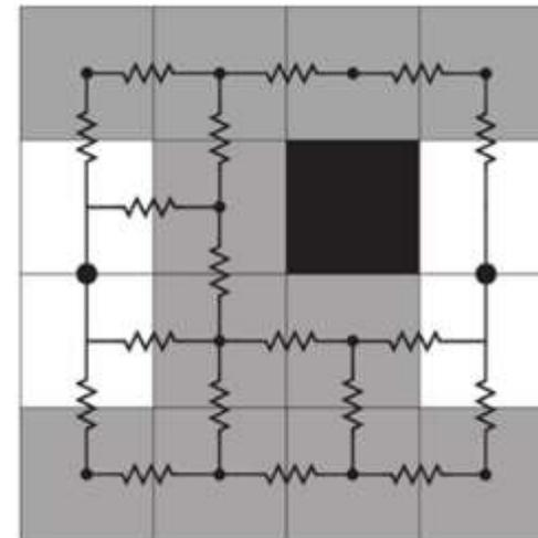
Every grid cell with finite resistance is represented as a node connected to neighboring cells. Cells with infinite resistance are dropped. Cells with 0 resistance are short-circuited.
