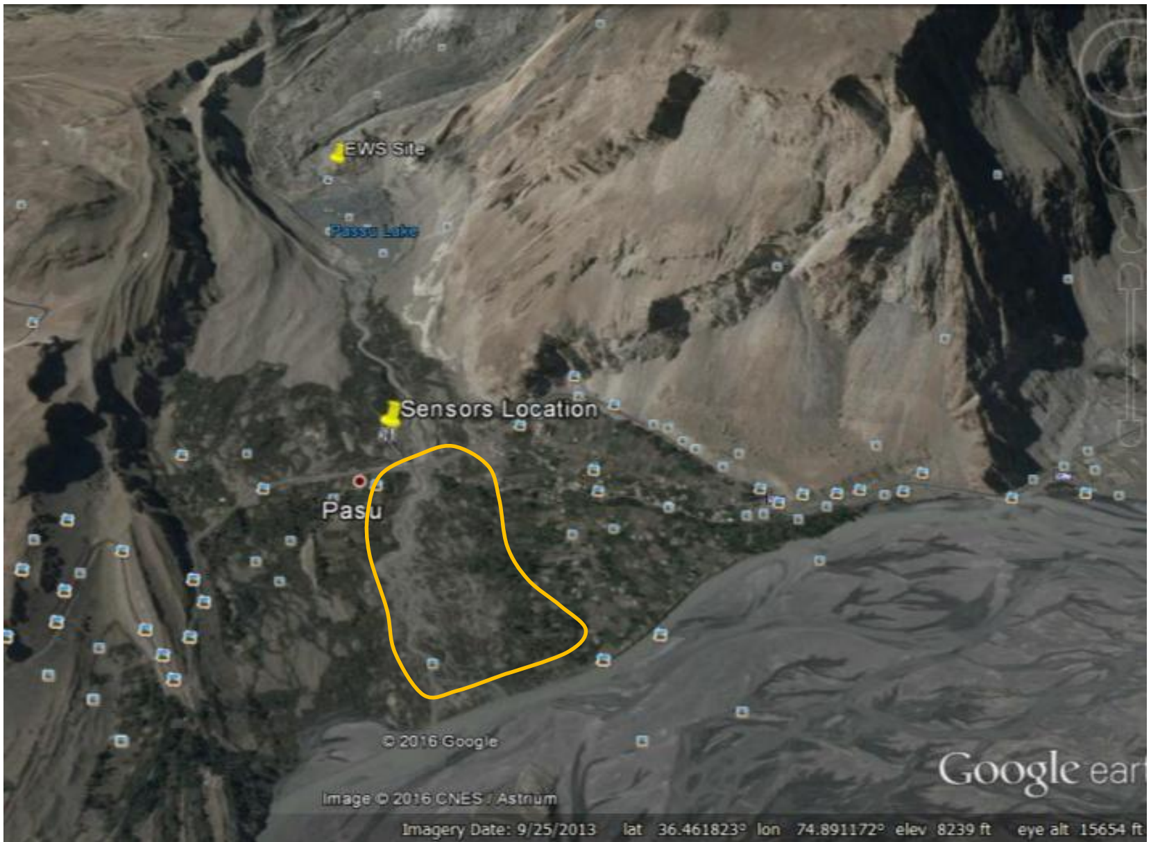
Fig4: The yellow polygon indicates the risky houses holds almost 21, yellow pinpoint shows the possible location for sensors and EWS site indicates the location for radar early warning system, from where it can easily sensors the out coming flood the glacier. Passu terminal moraine lake can also be seen on the map.
