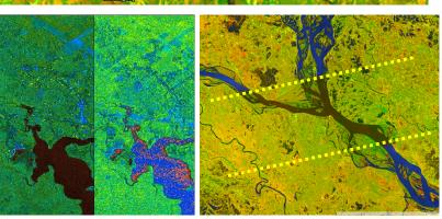
SAR RGBs can detect water – even through cloud cover but the methods are different from the passive measure used in optical images. In the following RGBS (left: SAR RGB; right: Sentinel-2 (S2) SWIR RGB; both from 2 Aug 20), water interpretation in the SAR image is reinforced by water seen in S2 image from the same day within 8 hours of SAR pass.
