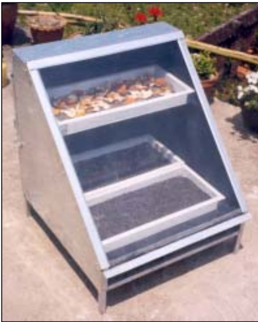
Locally manufactured solar dryer cabinet and apples dried in Jomsom District.
