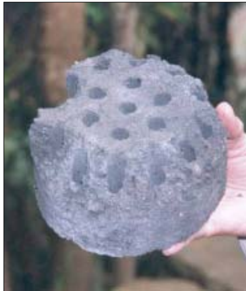
Poor quality briquettes disintegrate during transport.
