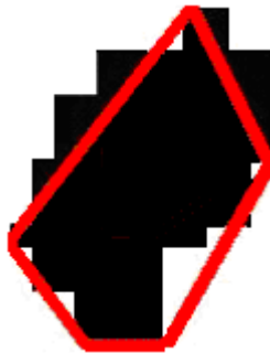
Figure 25.21. Raster image object (black area) with its polygon object (red lines) after vectorization
